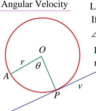
Let *O* be the centre of a circle, radius *r* units. If the point moves from *A* to *P* in time *t*, where  $\angle AOP = \theta$ , then the angular velocity,  $\omega$ , of the point is defined as the rate of change of  $\theta$  with respect to time.
