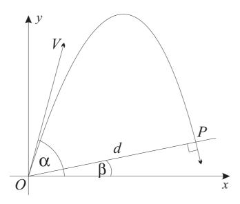
The diagram above shows the parabolic path of a particle that is projected from the origin O with velocity V at an angle of  $\alpha$  to the horizontal. It lands at the point P, which lies on a plane inclined at an angle of  $\beta$  to the horizontal. When the particle strikes the plane, it is travelling at 90° to the plane.
