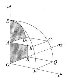
The solid in the diagram above has a horizontal square base OPQR with diagonal OQ = r. The thin horizontal slice ABCD at height z above the base is also square with OC = r. The line OA is vertical. The curve QCE is a quadrant of a circle with centre O and radius r.
