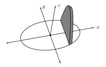
A certain dome tent is designed with an elliptical base  $\frac{x^2}{4} + \frac{y^2}{1} = 1$ , as in the diagram above. Cross-sections perpendicular to the base are segments of a parabola. The height of each parabolic segment is equal to the width of its base.
