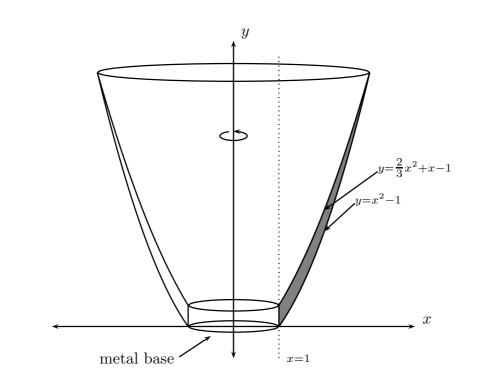
A glass is designed by rotating the region bounded by the curves  $y = x^2 - 1$  and  $y = \frac{2}{3}x^2 + x - 1$  and the line x = 1 about the *y*-axis, as in the diagram above. The resulting volume is to be grafted onto a cylindrical metal base whose volume need not be included in the following calculations.
