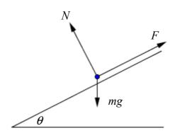
A particle of mass m is lying on an inclined plane and does not move. The plane is at an angle  $\theta$  to the horizontal. The particle is subject to a gravitational force mg, a normal reaction force N, and a frictional force F parallel to the plane, as shown in the diagram above.
