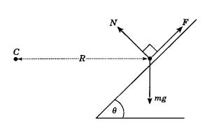
The reaction exerted by the track on the particle has a normal component N, and a component F due to friction, directed up or down the bank. The force F lies in the range  $-\mu N$  to  $\mu N$ , where  $\mu$  is a positive constant and N is the normal component; the sign of F is positive when F is directed up the bank.
