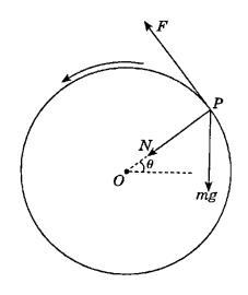
The centre of the drum is O, and OP makes an angle of  $\theta$  to the horizontal.
