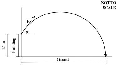
Assume that the equations of motion of the missile are  $\ddot{x} = 0$  and  $\ddot{y} = -10$
