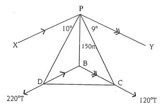
A ship is observed from the top of a 150m cliff *BP*. When the ship is at point *C* it has an angle of depression of 9° from the top of the cliff and later at D it has an angle of depression of 10°.
