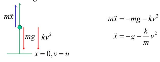
$$v\frac{dv}{dx} = \frac{-mg - kv^2}{m}$$
