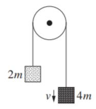
The force due to air resistance on each mass has magnitude kv, where k is a positive constant.
