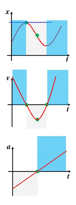
When displacement graph is stationary, velocity is zero
