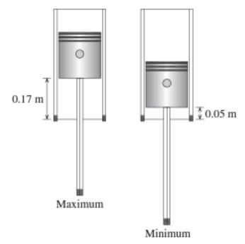
The mass of the piston is 0.8 kg. The piston completes 40 cycles per second.
